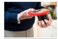
No power, no problem. Pull the cord. Generate electricity. Never run out of power. NowLight turns your effort into electricity. A minute of pulling will generate up to 2 hours of light or enough power for a 15-minute phone call. NowLight can also be charged from USB power sources or using a solar panel. Weblink.
